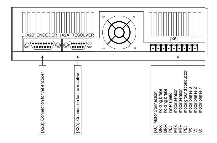
Figure 3: Servo positioning controller ARS 2102 FS: Bottom view
