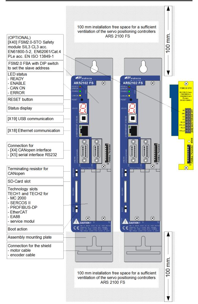
Figure 1: Servo positioning controller ARS 2100 FS: Front view and Installation space
