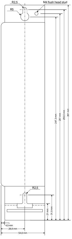
Figure 4: Servo positioning controller ARS 2100 FS: Mounting plate
