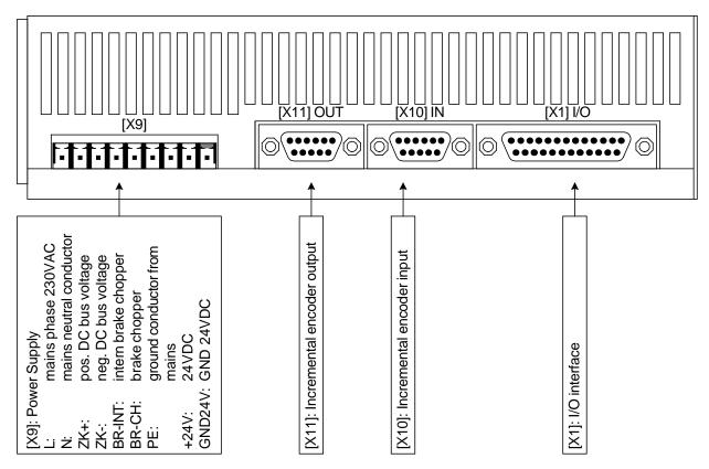
Figure 2: Servo positioning controller ARS 2102 FS: Top view
